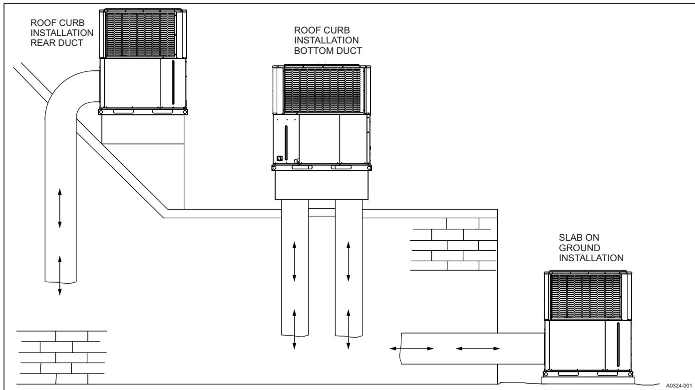
**UNIT TYPICAL SLAB ON GROUND INSTALLATION**
